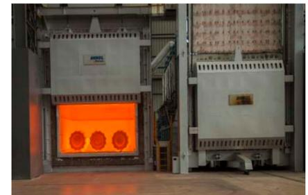
30 MT Chamber gas fired reheating furnace from Andritz Metals, Germany
