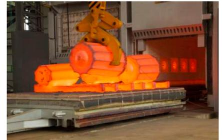
40 MT Car bottom gas fired reheating furnace from Andritz Metals, Germany
