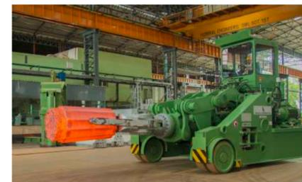
14 Ton Tyre Bound Forging Manipulator from Dango & Dienenthal, Germany
