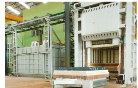
5 MT Car Bottom Electrically Heated Furnace from Andritz Technologies, India and 10 MT Chamber Electrically Heated Furnace from Wesman Engineering, India
