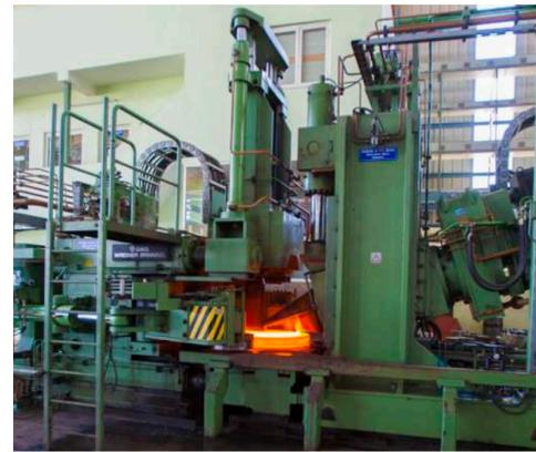
Radial-Axial Ring Rolling Machine from SMS Meer GmbH, Germany
